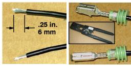
6. Connect brake wires to new connector (non-polarity sensitive). Wire terminals should snap into position. Install secondary lock.
