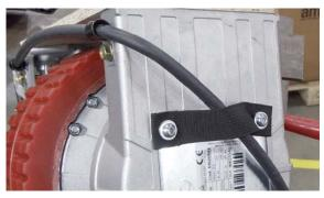
11. Connect jumper harness to the main machine harness and secure connectors to stabilizer bar with wire-ties as shown. Replace existing harness clamp with smaller clamp as shown.
