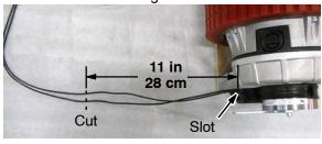
Strip brake wires as shown. Using the Packard crimping tool, install new terminals and seals to wires as shown.
