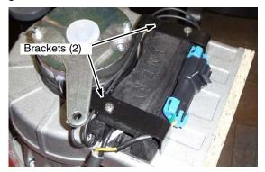
9. Secure jumper harness with smaller harness clamps supplied with kit.
